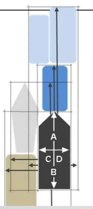
Dimension field can now be used to represent the a vessels tow (type22)
